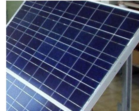
Silicon Nitride formed with PECVD, color is dark blue which is good for absorbing more sun power. The conversion efficiency is of one highest worldwide.
